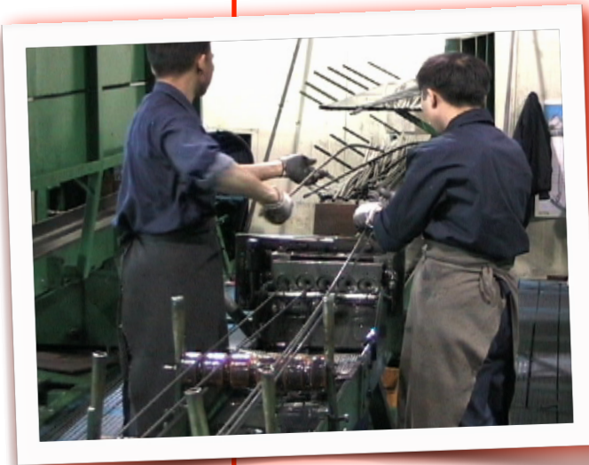
Yunan workers feed 1" aluminum tubing to be "pultruded" down to 13mm, pickled, straightened, and anodized to give its beautiful and statin finish.
